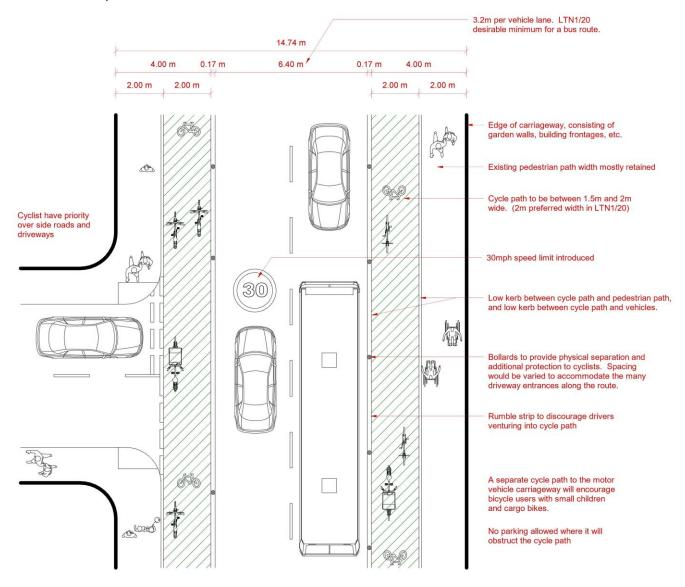
The next plan shows an example of one of the pinch points with segregated cycle, pedestrian and vehicle lanes which can be provided for by reducing lane widths, speeds and prohibiting overtaking. The pinch points are all about 11m, under the required width for full-width cycle lanes.
